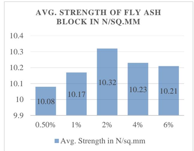
Fig. 3: Avg. Compressive Strength vs. PET Fibers
