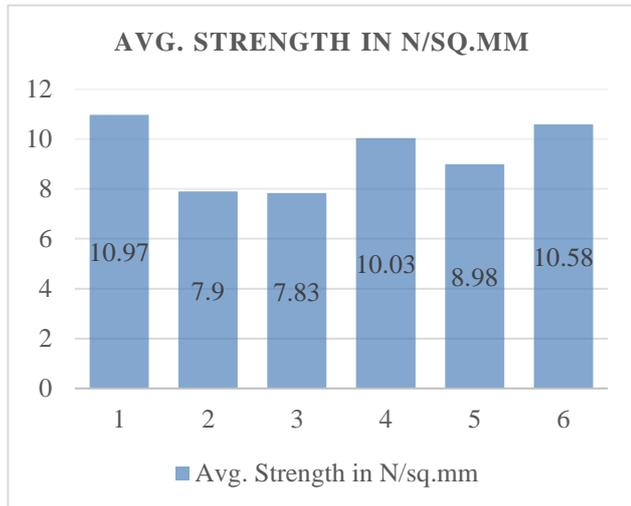
Fig. 2: Avg. Compressive Strength Vs. Different Types of Cores
