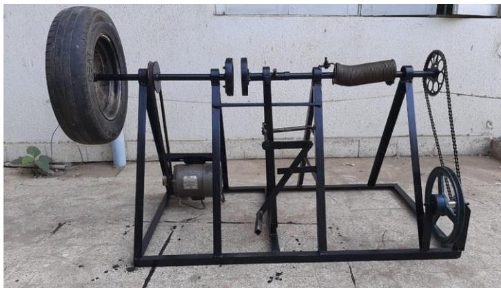
*Fig. 1:-assembly of flywheel based regenerative braking system*
